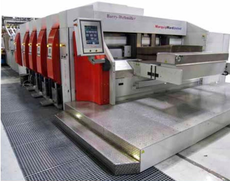
Ideally suited to P-Well's requirements: The combination of robust machine construction from MarquipWardUnited and highly modern control technology from B&R results in a new rotary die machine with very high throughput.
