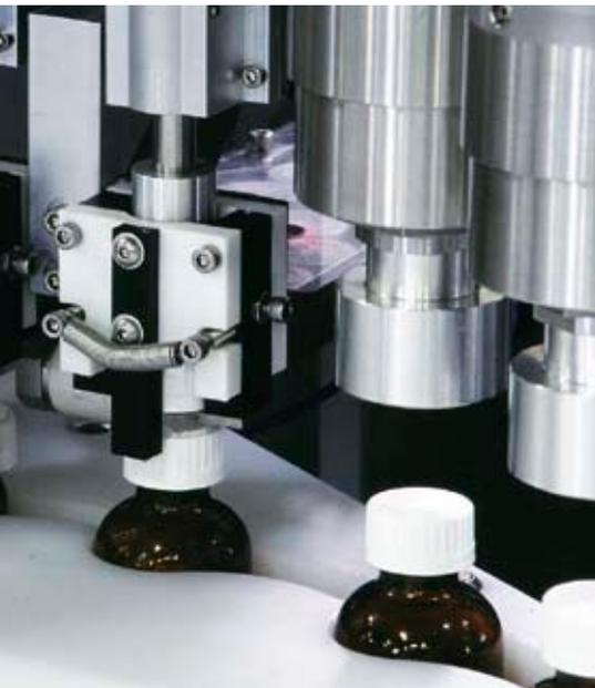
After the bottles enter the system they are then fed into a servo-driven timing screw, which controls the position of the bottles for the filling process.
