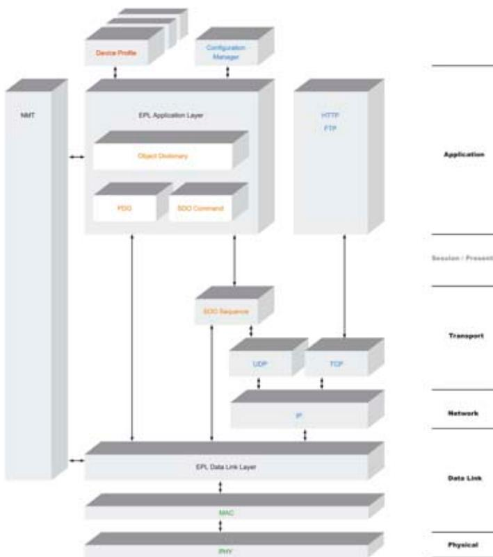
The ETHERNET Powerlink protocol stack is based on established international standards.
