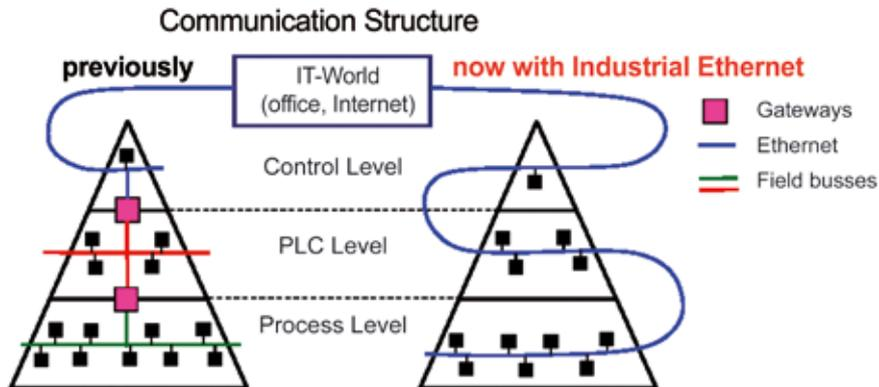
Industrial Ethernet promises a standardized networking environment from the control level down to the process itself.
